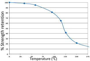
TA4302 can withstand higher temperatures for brief periods (such as for paint baking and wave soldering processes) providing the joint is not unduly stressed. The minimum temperature the cured adhesive can be exposed to is -40°C (-40°F) depending on the materials being bonded.
