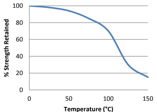
“Hot strength” shear strength tests performed on glass to mild steel. Fully cured specimens conditioned to pull temperature for 30 minutes before testing at temperature.
