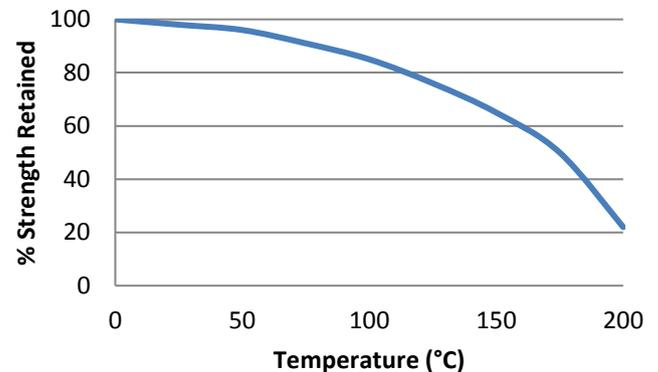
"Hot strength" shear strength tests performed on mild steel. Fully cured then conditioned to pull temperature for 30 minutes before testing.
