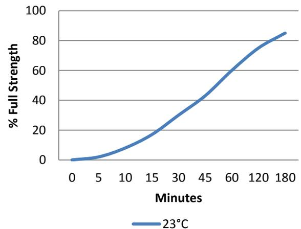
Graph shows typical strength development of bonded components. An increase of temperature may result in a faster cure; lower temperatures may give a slightly slower cure.
