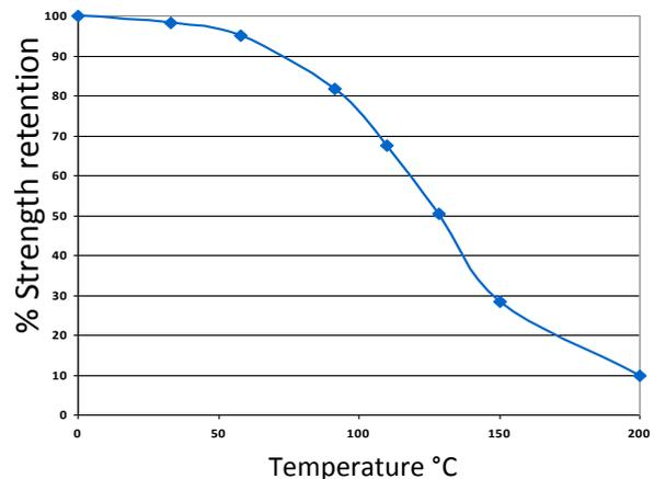
4UV80HV can withstand higher temperatures for brief periods (such as for paint baking and wave soldering processes) providing the joint is not unduly stressed. The minimum temperature the cured adhesive can be exposed to is -55°C (-67°F) depending on the materials being bonded.
