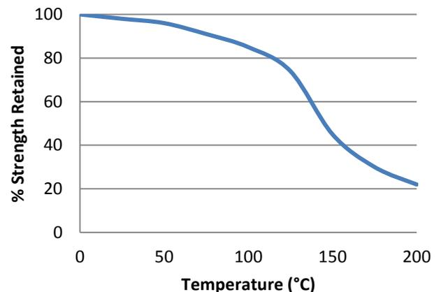
“Hot strength” shear strength tests performed on mild steel. Fully cured then conditioned to pull temperature for 30 minutes before testing. ES5741 can withstand higher temperatures for brief periods (such as for paint baking and wave soldering processes) providing the joint is not unduly stressed. The minimum temperature the cured adhesive can be exposed to is -40°C (-40°F) depending on the materials being bonded.
