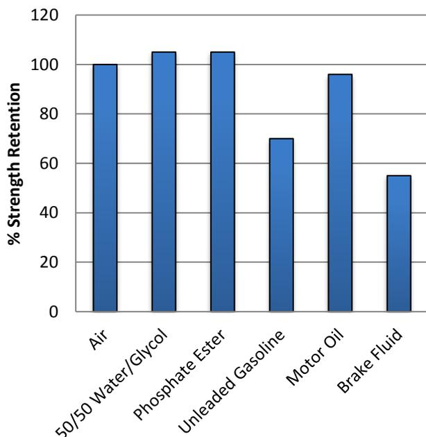
Specimens were immersed for 30 days at 85°C and tested at room temperature.
