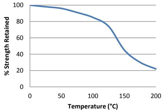
“Hot strength” shear strength tests performed on mild steel. Fully cured then conditioned to pull temperature for 30 minutes before testing. ES578 can withstand higher temperatures for brief periods (such as for paint baking and wave soldering processes) providing the joint is not unduly stressed. The minimum temperature the cured adhesive can be exposed to is -40°C (-40°F) depending on the materials being bonded.
