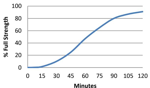
Graph shows typical strength development of bonded components at 23°C. Curing at higher or lower temperatures may affect cure speed.
