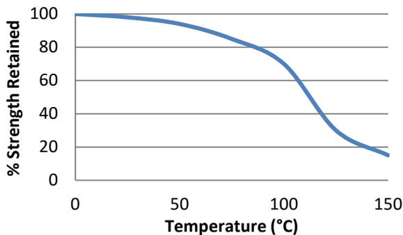
“Hot strength” shear strength tests performed on mild steel. Product fully cured at room temperature and conditioned to pull temperature for 30 minutes before testing.
