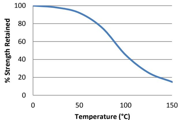
“Hot strength” shear strength tests performed on mild steel. Fully cured then conditioned to pull temperature for 30 minutes before testing. MS359 CLEAR can withstand higher temperatures for brief periods (such as for paint baking and wave soldering processes) providing the joint is not unduly stressed. The minimum temperature the cured adhesive can be exposed to is -40°C (-40°F) depending on the materials being bonded.
