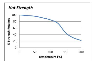
then conditioned to pull temperature for 30 minutes before testing. ES569 can withstand higher temperatures for brief periods (such as for paint baking and wave soldering processes) providing the joint is not unduly stressed. The minimum temperature the cured adhesive can be exposed to is -40°C (-40°F) depending on the materials being bonded.
