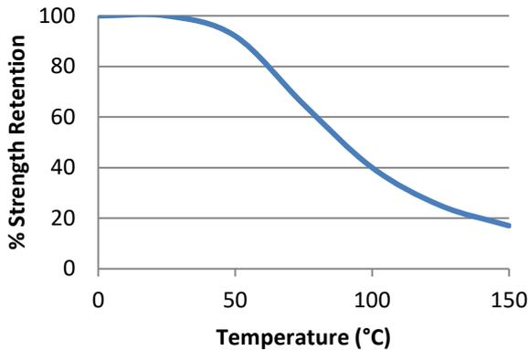
"Hot strength" shear strength tests performed on mild steel. Fully cured specimens conditioned to pull temperature for 30 minutes before testing at temperature.
